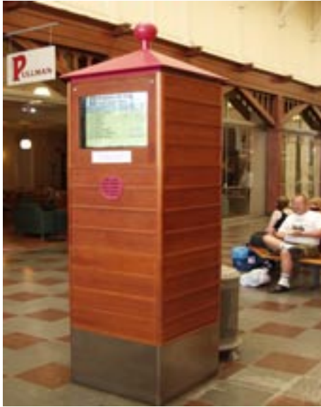
Figure 2: At the Central Station in Göteborg a computer screen is built into a tower to make the display more aesthetically pleasing.
